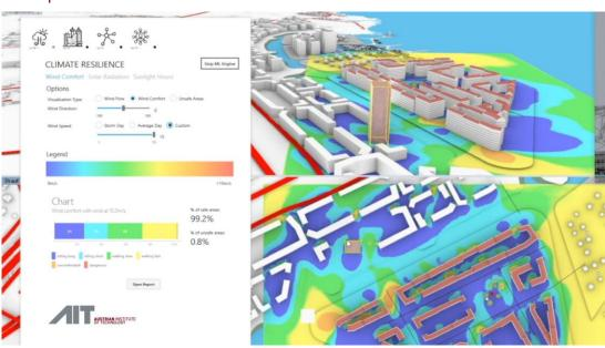
The researchers of the City Intelligence Lab of the AIT Center for Energy developed a wind simulation that can determine wind factors in planning within seconds. © AIT
