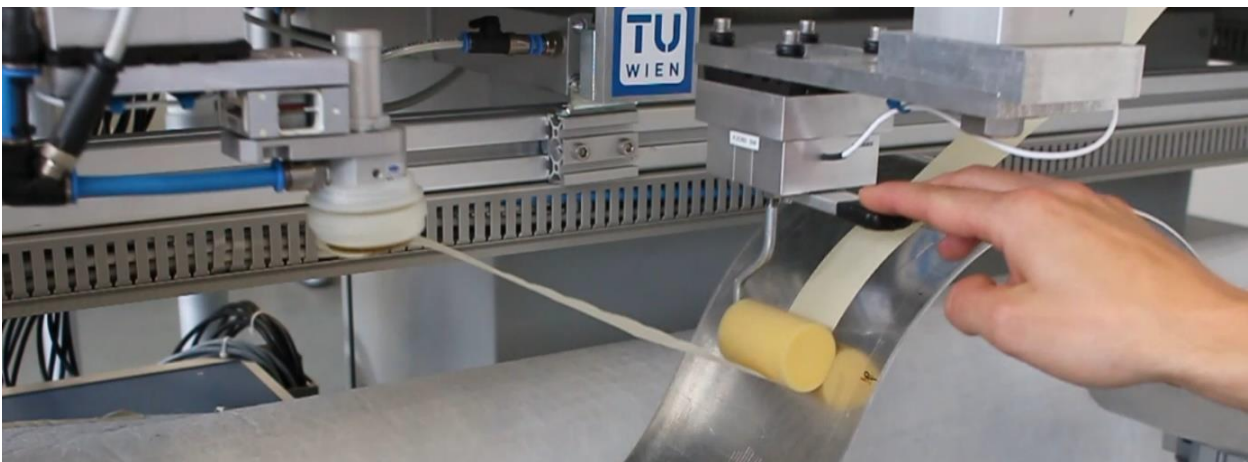
Figure 2: Cooperation between man and machine when applying an adhesive strip. © Stefan Flixeder
